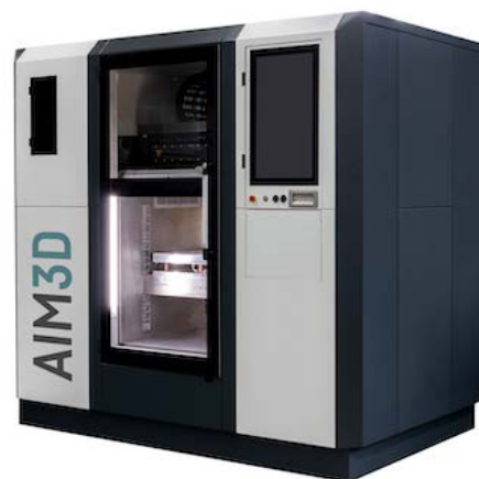
The ExAM 510 is suitable for metals, ceramics and polymers (Courtesy AIM3D GmbH)
